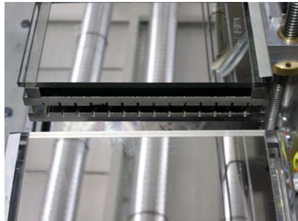
Figure 5: View of neutron guide element 3 with its upper channel used for continuing NL-2b (height: 12 mm; width: 170 mm) and its lower channel designed as a radial pre-collimator.
