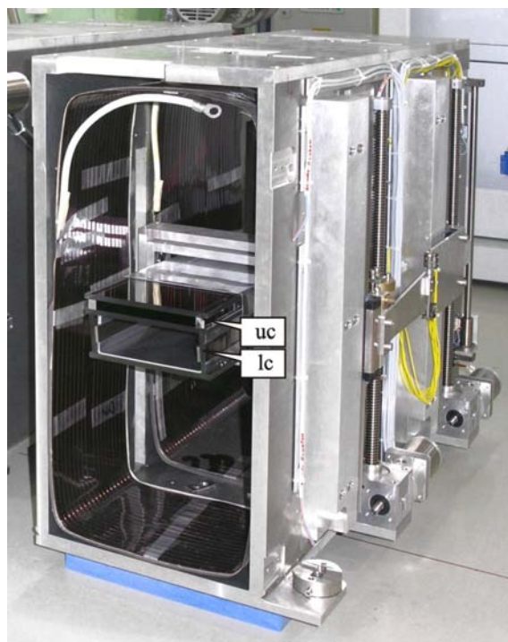
Figure 3: View of a neutron optical body of the beam guide chamber with the mechanics for vertically aligning a NGE. The NGE consists of an upper channel (uc) for continuing NL-2b (height: 12 mm; width: 170 mm) and a lower channel (lc) designed for vertically collimating and keeping the large horizontal beam divergence.
