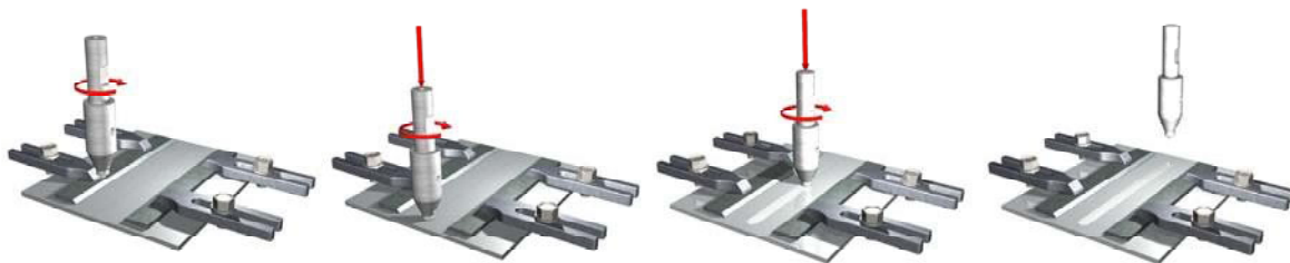
Figure 1: Schematic of FSW process: Left to right: tool rotation, tool plunge, tool traverse, tool exit.
