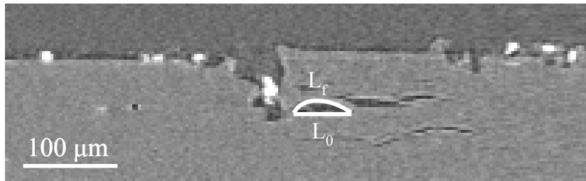
Figure 3: A spall created by the impact is evident and used to estimate the fracture strain.
