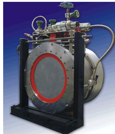
Fig.1: Schematic view and photo of the thermal neutron detector
