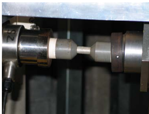
Fig. 1: AZ 31 Cylinder (30mm x 10 mm Ø) in FSS stress rig (RT Experiment)
